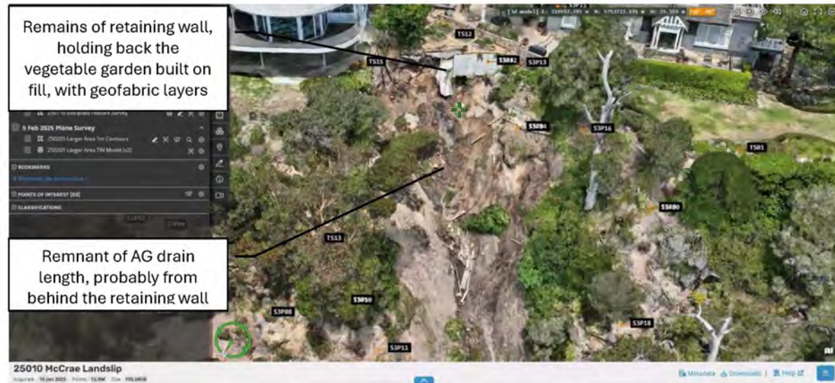
Figure 14: Drone footage showing detail of the failure.
