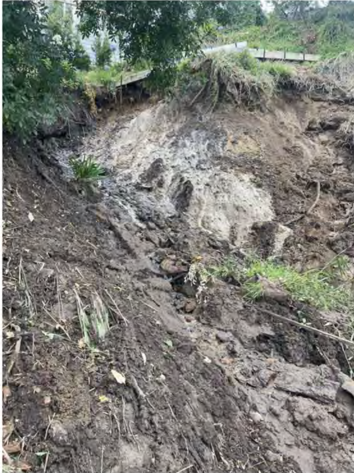
Figure 56: Photograph taken on 6 January 2025, looking up at the landslide, showing saturated debris flow surface with dry soil adjacent. Debris may include some boulders cobbles, but also anthropogenic and vegetation material
