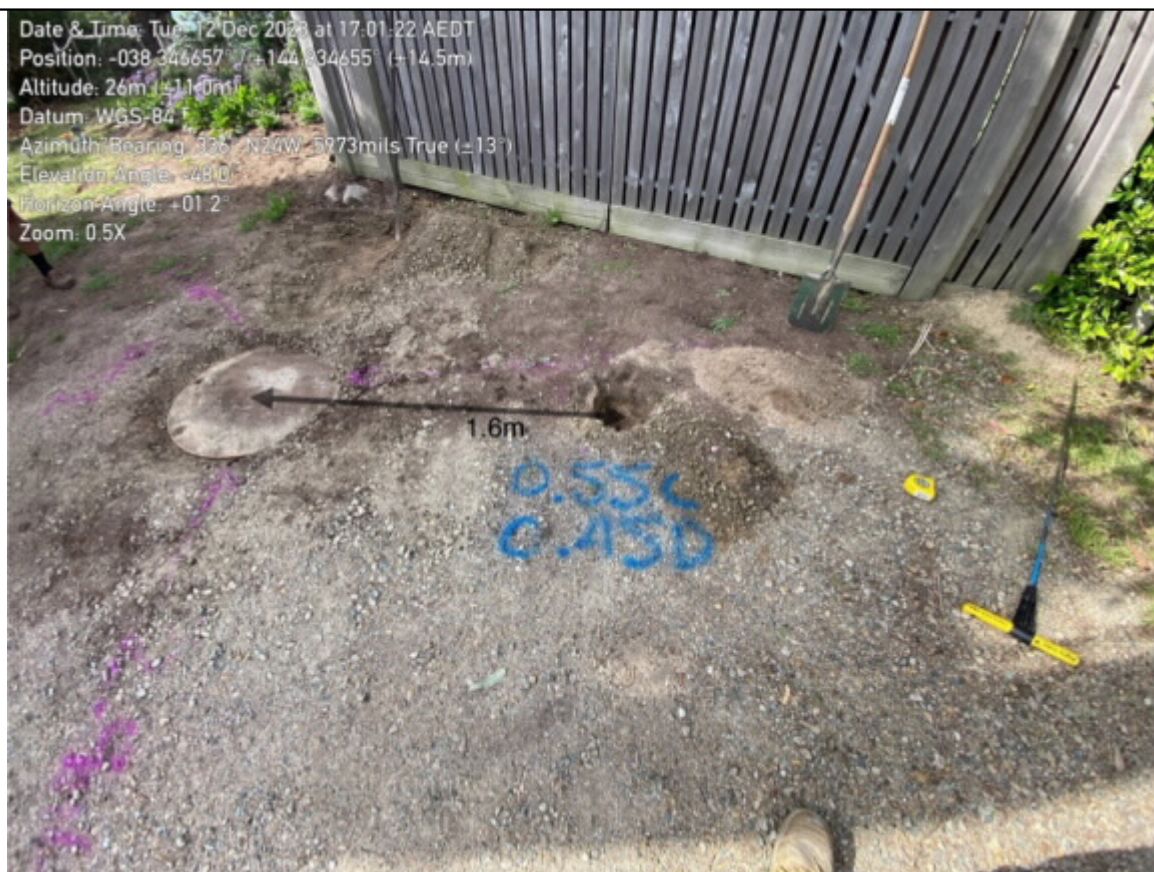
Fig 3: Scan validation location, positioned to avoid underground utilities. Void was proven with 0.55m cover.
