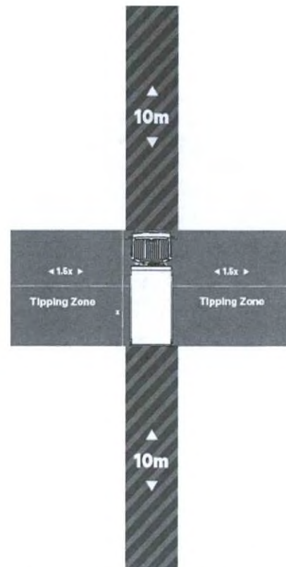
Figure 1. The Red Zone for Tipper trucks, designed to prevent plant / pedestrian injuries
