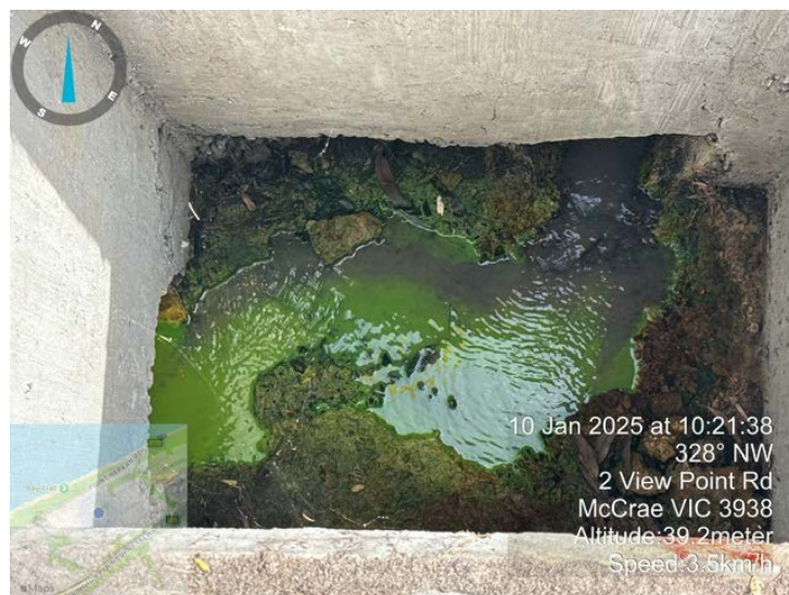
Photo 5: Inspection Pit Corner Prospect Hill Road and View Point Road waiting for red trace dye to appear.
