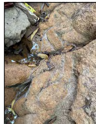
Photo 33B - Exposed XW Granite at invert of Coburn Avenue creek (02/04/2025)
