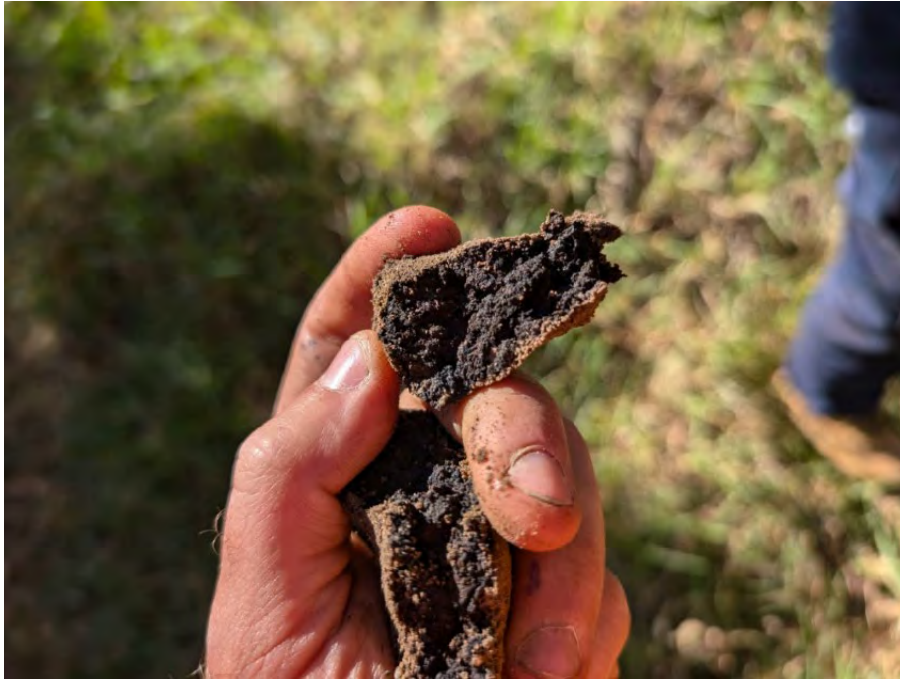
Inset 40: Inferred Gully Alluvium encountered at NDT14A
