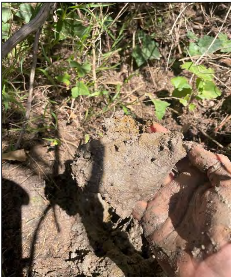
Photo 13 - Saturated soils immediately North-East of stairs on 10-12 View Point Road (24/01/2025)
