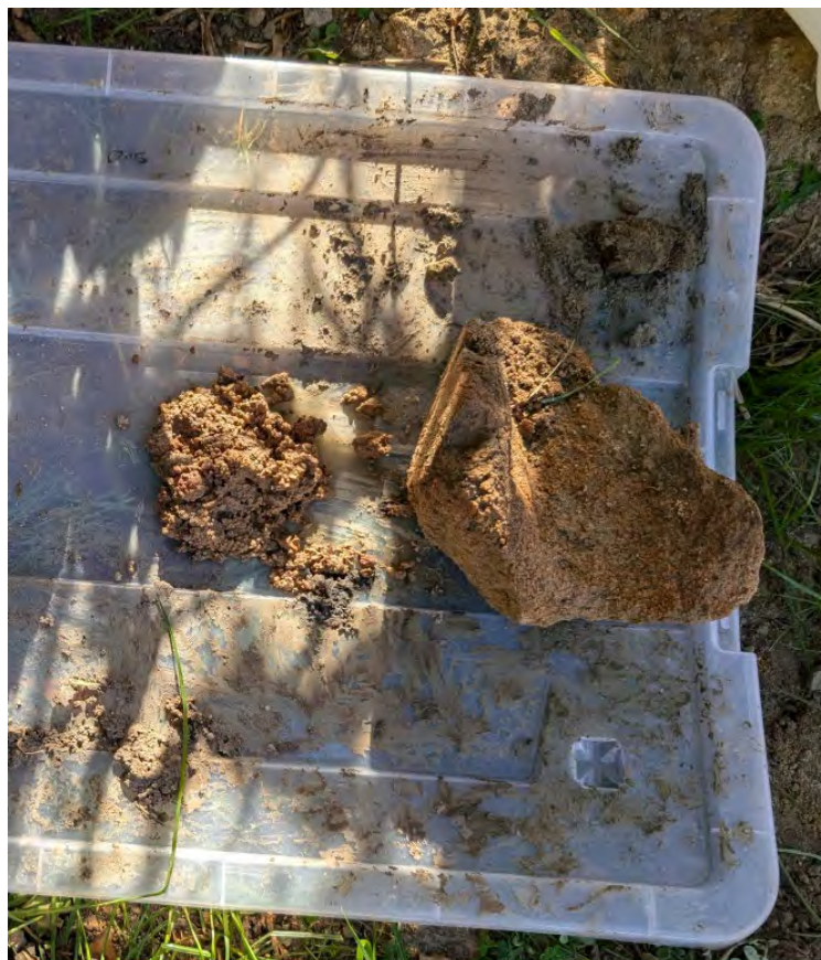
Inset 38: Inferred Colluvium recovered from NDT13 showing SAND and a BOULDER
