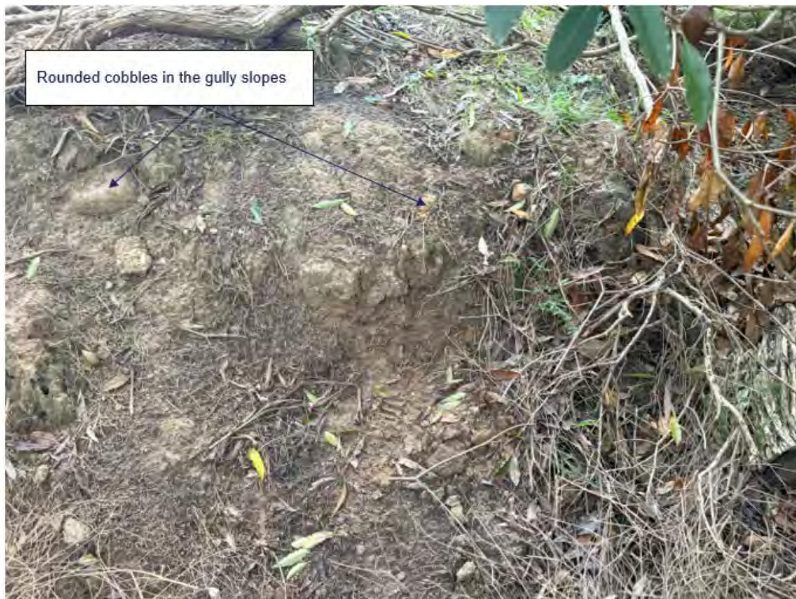
Inset 39: Inferred Colluvium at surface of the gully between Bayview Road and MPF. Refer to Inset 27 for location.
