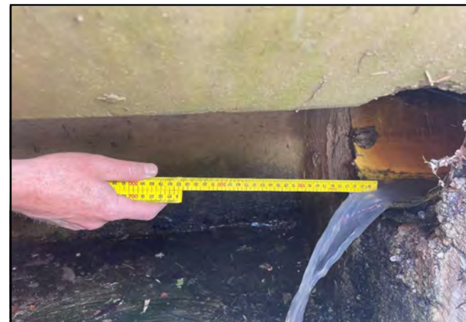
Photo 2 - Depth of flow in View Point Road stormwater (06/01/2025)
