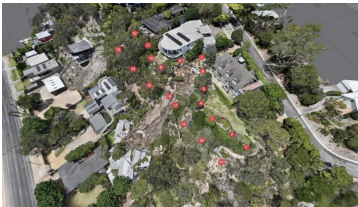
Figure 1 – Indicative layout of tilt sensors over the slope, to be confirmed and refined under the direction of geotechnical SME. Prisms to be installed on tilt sensor locations to provide 3D displacement calibration of tilt data.
