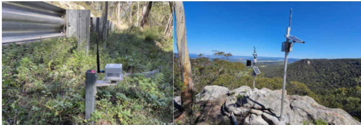
Figure 2 - an omni tilt sensor (left) installed on a roadside embankment, reporting tilt data to the 4G Gateway (right) which uploads the data to the cloud monitoring portal for visualisation and alerts.
