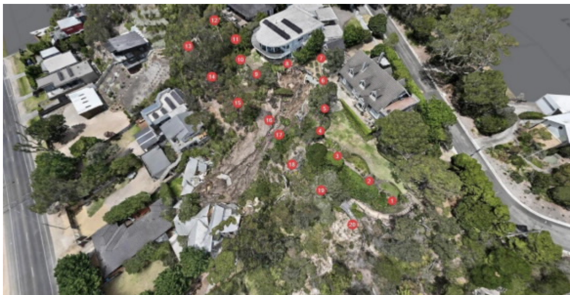
Figure 1 – Indicative layout of tilt sensors over the slope, to be confirmed and refined under the direction of geotechnical SME. Prisms to be installed on tilt sensor locations to provide 3D displacement calibration of tilt data.
