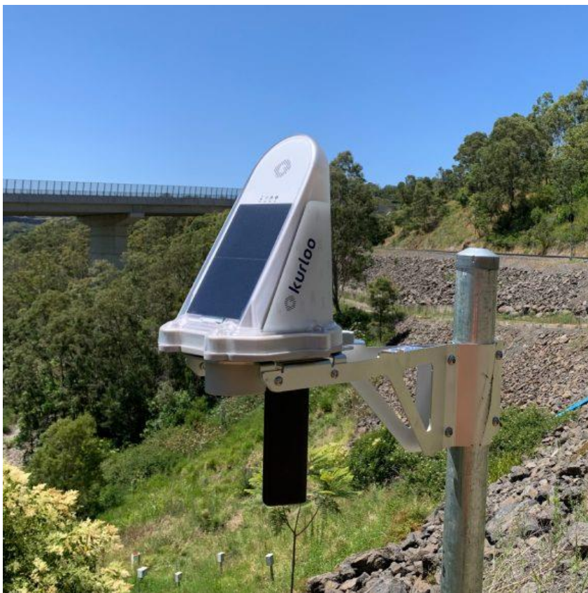
Figure 1: Example of GNSS Sensor installed on steel post
