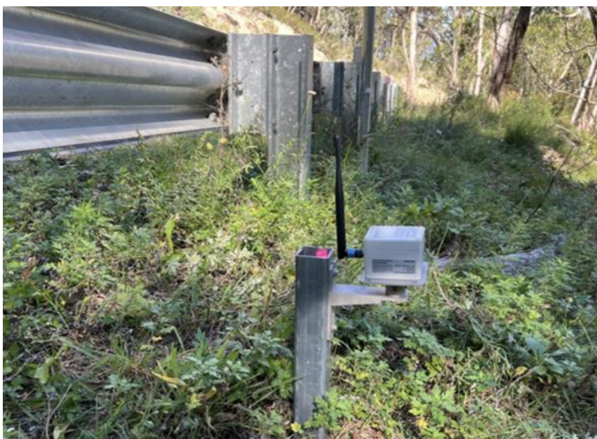
Figure 2: Example of tilt sensor installed on steel post
