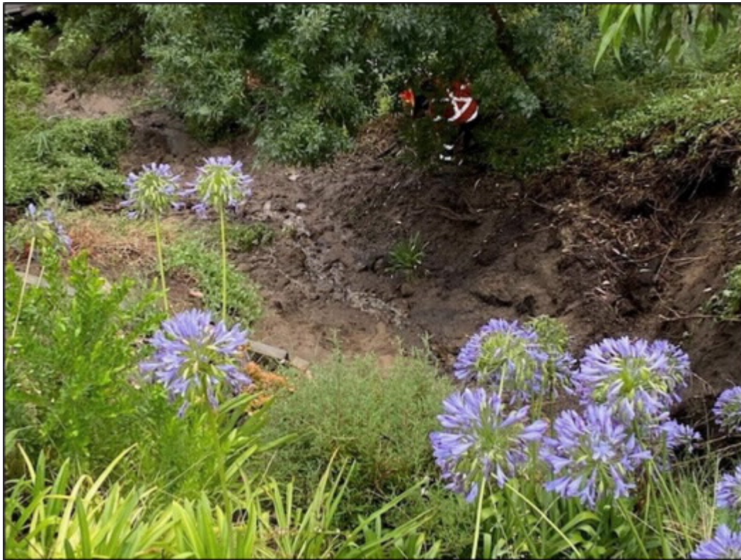
Photograph 2: Water flow observed downslope of 6 January 2025 landslide, originating from base of landslide headscarp
