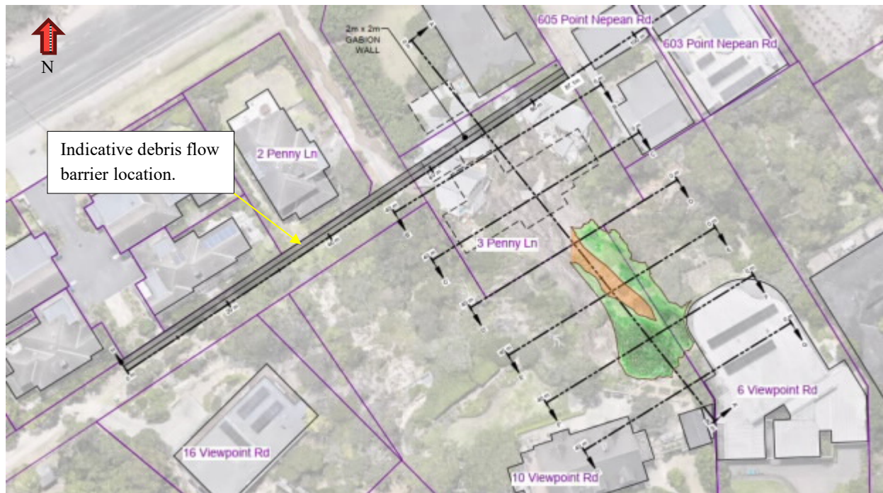
Figure 9.5 Indicative location for bund to intercept debris flowing to base of escarpment.
