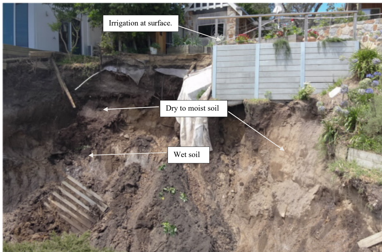
Figure 8.13 Photo of headscarp following January 14 landslide with areas of dry and wet ground annotated. PSM.5000.0001.0290, photo dated 15th January 2026.
