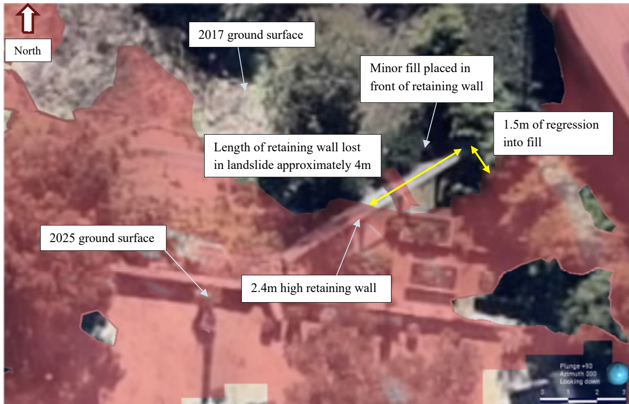
Figure 7.11 Comparison of 2017 and 2025 ground surface showing proportion of retaining wall and fill evacuated during the landslide.
