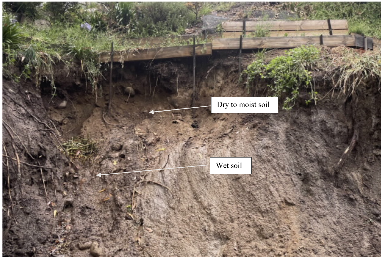
Figure 8.12 Photo of headscarp following 5 January 2025 landslide with areas of dry and wet ground annotated. PSM.50000.0001.0114, photo dated 6 January 2025.
