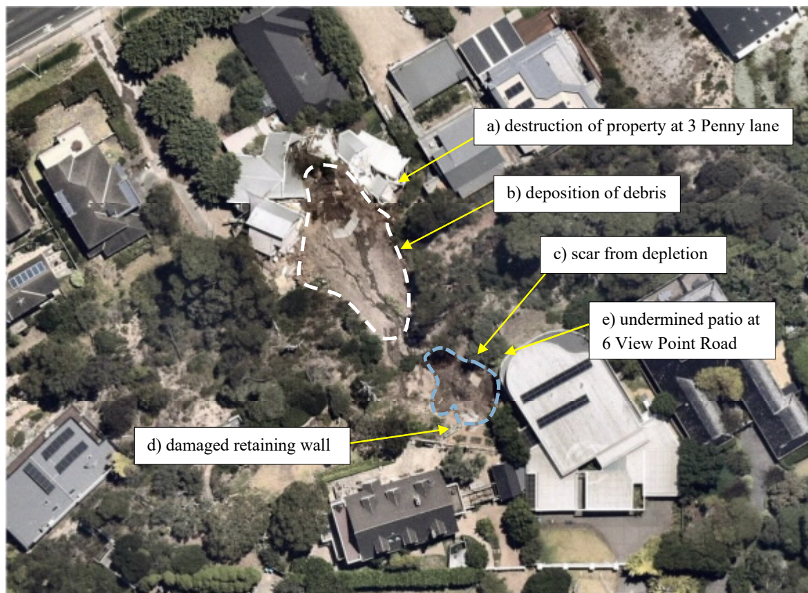
Figure 9.1 Annotated plan showing key damage caused by the 2025 landslide
