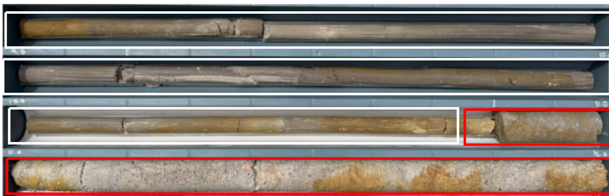
Figure 6.6 Core recovered from BH01 showing residual soils (white) and extremely weathered granite (red). Depth range 8 m to 12 m below ground surface.
