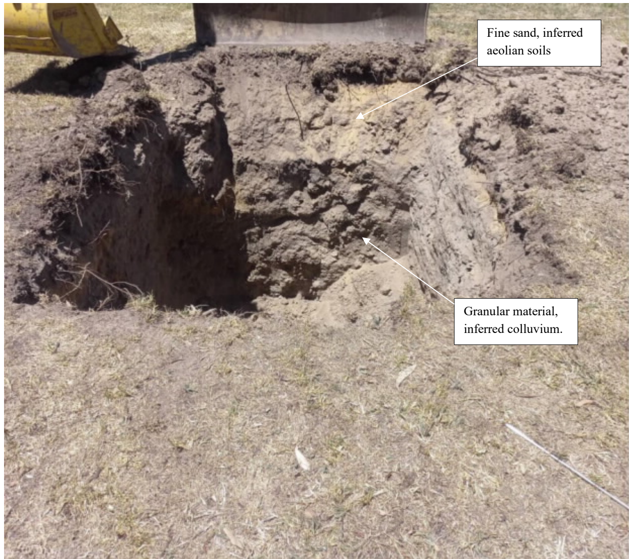
Figure 6.11 Transported soils exposed on Bayview Road opposite The Boulevard Reserve (SME.0001.0001.0120)
