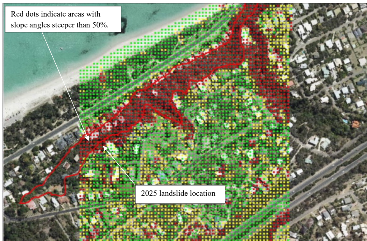
Figure 7.18 Extract from Lane Piper 2012 report showing assessed landslide susceptibility on the McCrae escarpment, with my annotations added.
