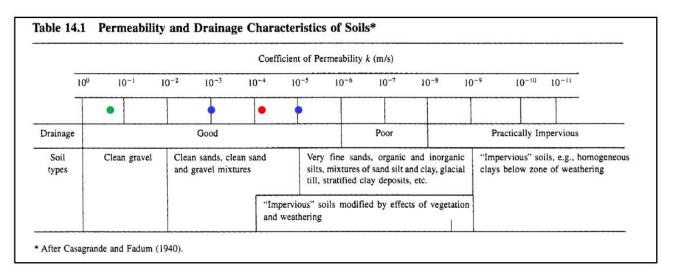
Inset 5: Excerpt from Terzaghi et al (1996) – Permeability with mark up of SMEC estimate (red) and WSP estimate (blue) and WSP interpretation of dye test at NDT01 (green).
