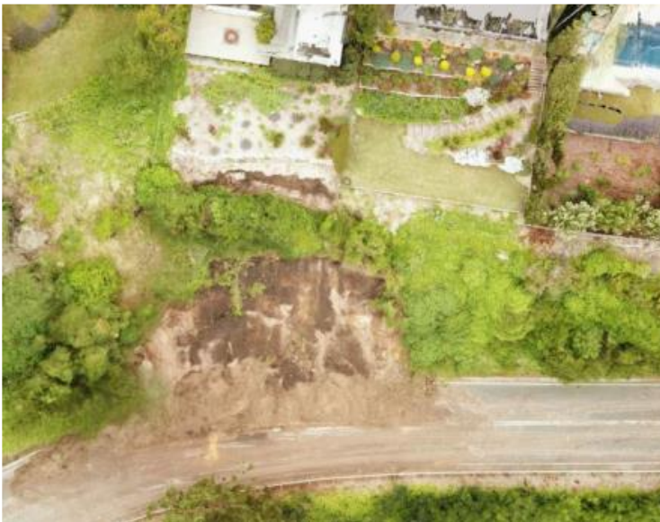
Figure 4 Collapsed Slope Prior to Stabilisation
