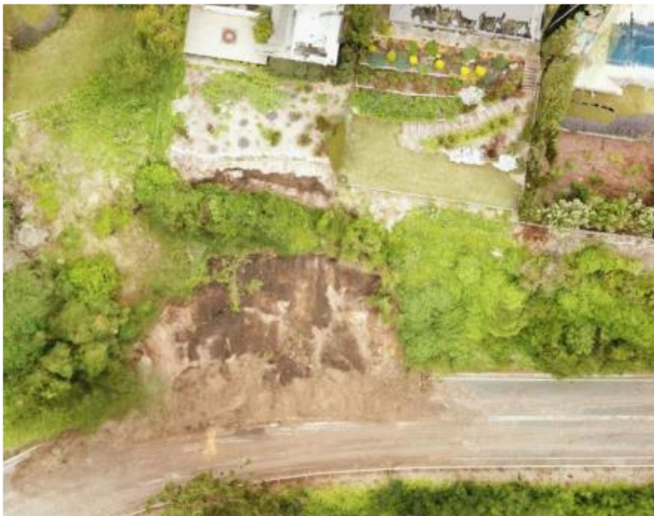
Figure 4 Collapsed Slope Prior to Stabilisation
