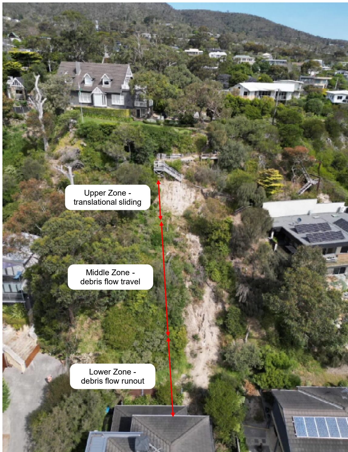
Photo 3 - Landslide Overview, with zones indicated
