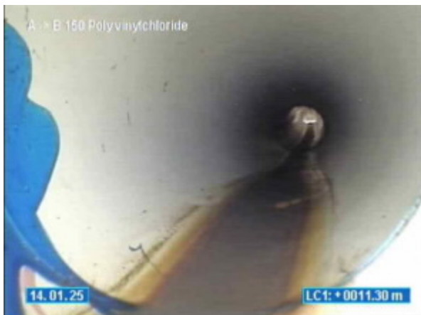
10-12 VIEW POINT ROAD MCCRAE_15.01.2025_090054_A TOO B _007.jpg, 00:03:24, 11.30 Inspection (survey) abandoned, Line deviates
