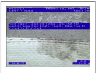
Location of Observation: 31.52m Video Position: 00:05:16 Observation Code: RPL Point repair, localised lining--less than the complete inspection length, length: 600mm from 12 o'clock to 12 o'clock
