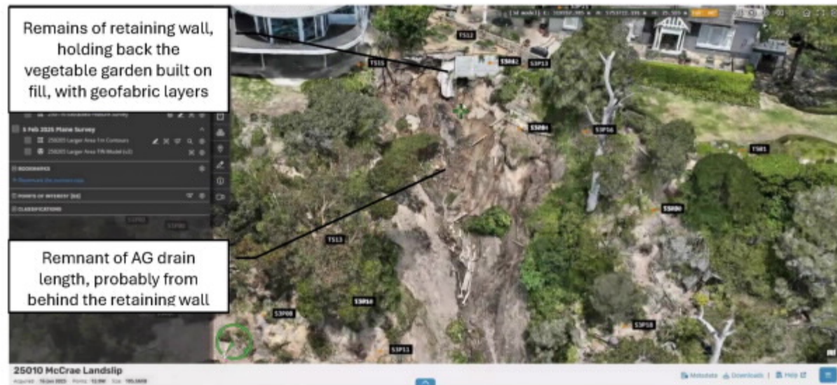
Figure 14: Drone footage showing detail of the failure.
