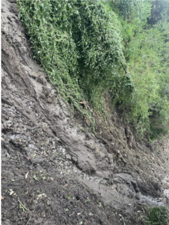
Figure 55: Photograph taken on 6 January 2025, showing slip debris of the 5 January 2025 landslide and water channel cutting through debris. The adjacent vegetation may indicate the original ground level and vegetation cover prior to the failure.
